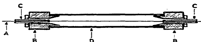
Fig. 2. Section of proportional counter. A: Tungsten wire 0.002 in. diameter. B: Polythene plug. C: Brass insert. D: Copper tube \frac{1}{2} in. diameter.
